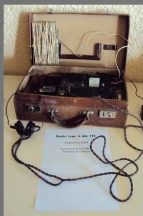
Radio type A MK III, 1944 3-9MHz, 5W _ Angleterre
