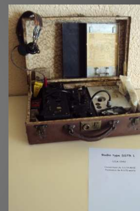
Radio type SSTR I, 1942 3-14MHz, 8-15W _ USA
