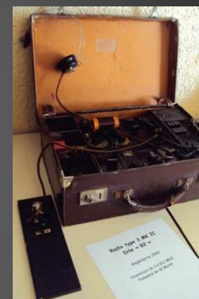
Radio type 3 MK II, 1942 3-15MHz, 18W _ Angleterre
